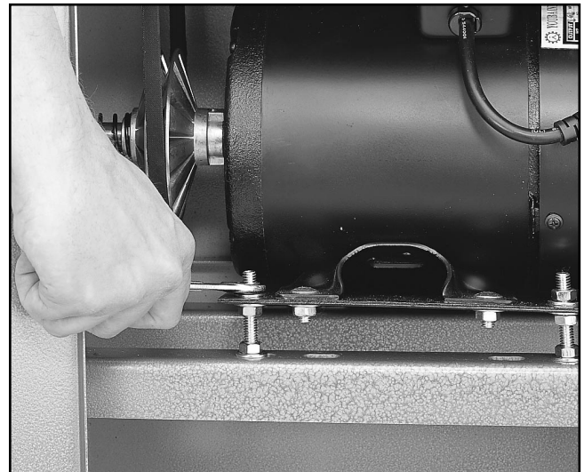
Figure 7. Loosening motor mount bolts.
